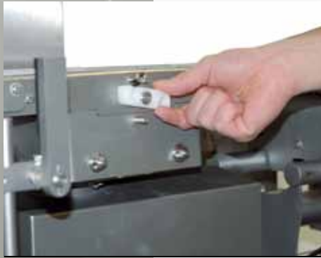
The quick-release conveyor fasteners ...
