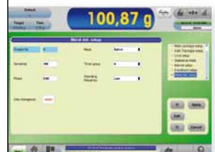
Operation of the optional metal detector occurs entirely on the weighing terminal
